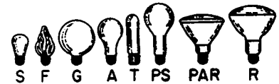
Fig. 12.5.2 Typical filament lamp shapes: S, straight; F, flame; G, globe; A, general service; T, tubular; PS, pear shape; PAR, parabolic; R, reflector.
